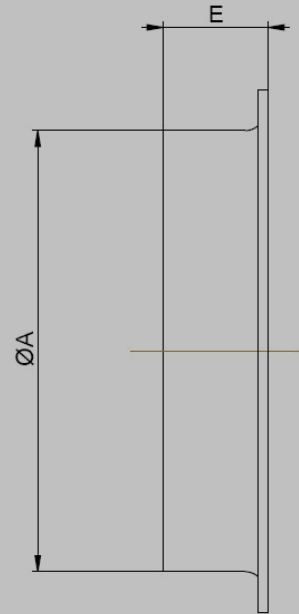
BA—BH Air inlet in cylindrical shape
